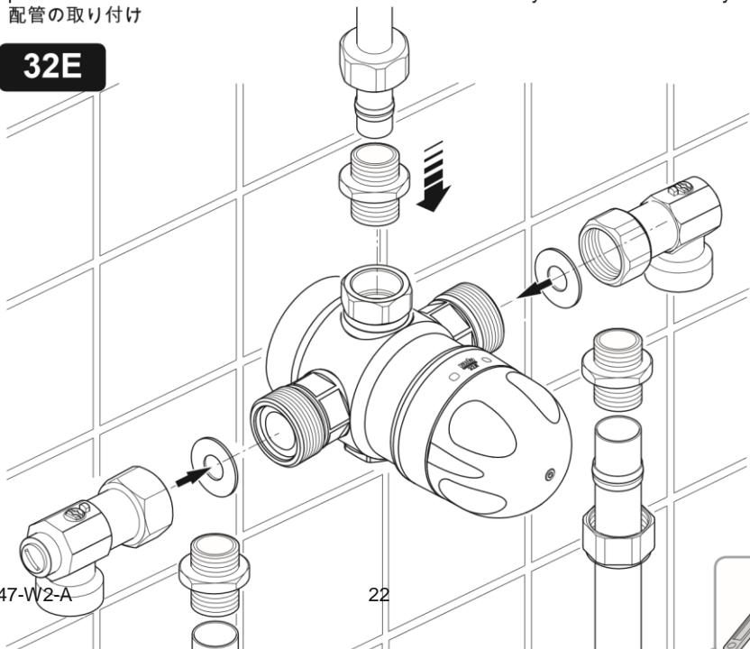
32E shown. The rest of the installation procedure is similar for all variants of the 32 valve.
