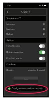
A notification as shown in the image (left) indicates that the product is successfully configured with new settings.
