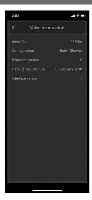
The Valve Information sub-menu provides detailed diagnostic information of the product, useful for fault finding and traceability for servicing.
