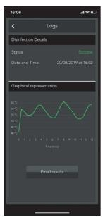
The summary report will appear indicating either a "Success" or "Fail" of the thermal disinfection cycle against the specified configured temperature limit. A date / time stamp will also be applied to the log. The log can be emailed from your mobile device for record-keeping purposes.
