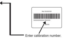
Caution! The valve must be calibrated if either the mixing valve assembly or the DMV control PCB are replaced. The calibration number is required for optimum performance and this can be found on the mixing valve body as shown above.
