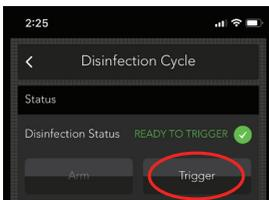
3 The message "Ready to Trigger" will appear once the product has acknowledged the request. Tap "Trigger" to confirm and initiate the disinfection cycle within 30 seconds of arming. Failure to trigger will require the Arm process to be repeated.
