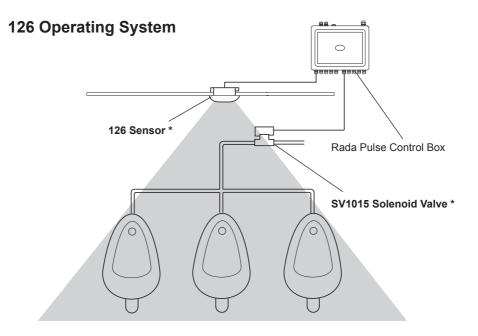
**Note!** Only the Sensor and Solenoid are supplied with this operating system as indicated \*
