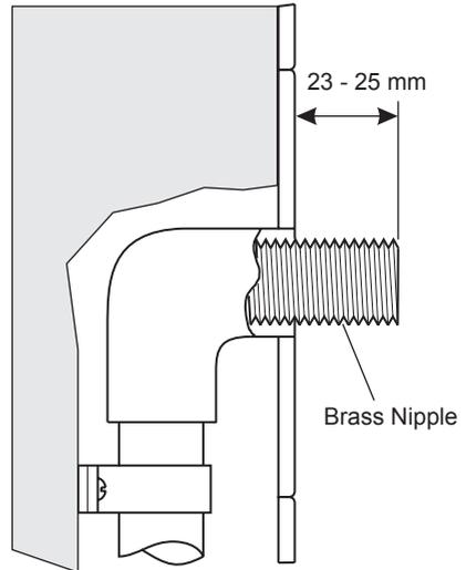
4. Place the wallplate over the brass nipple. Make sure that the foam seal is fitted against the finished wall surface.
