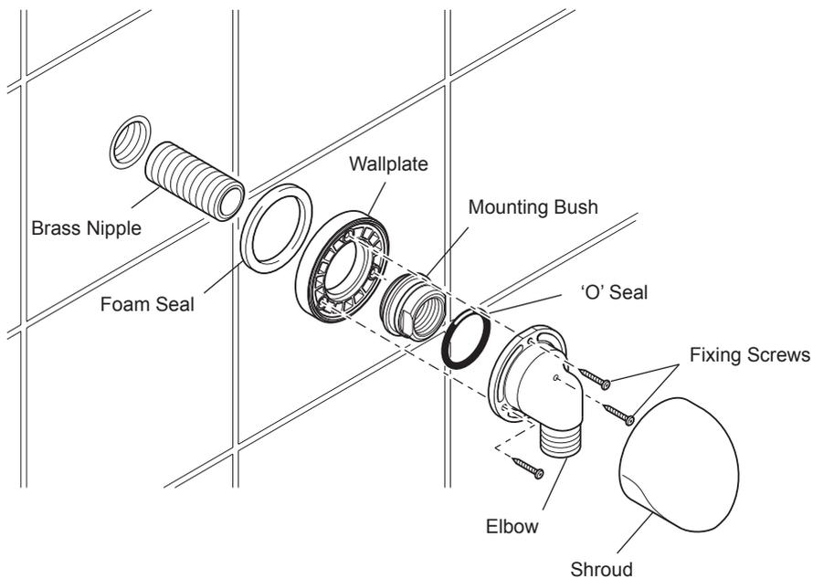
9. Push the elbow fully on to the mounting bush and secure with the three fixing screws.
