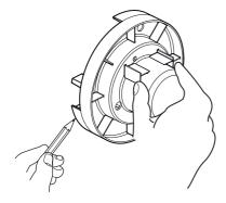
Mark the routes for the hot and cold supply pipework (Hot - Left, Cold - Right) and for the outlet pipework.
