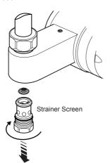
The non return valve cartridge and/or strainer screens can be cleaned or replaced as necessary.
