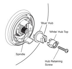
Once the desired maximum blend temperature has been achieved, refit the 'blue' hub without disturbing the spindle.
