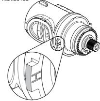
**Note!** Should the supplies be reversed then the mixing valve will not be able to control temperature. This can be corrected by rotating the thermostatic cartridge within the valve body, refer to section: 'Installation, Outlet Position/ Reversed Inlet Supplies'.
