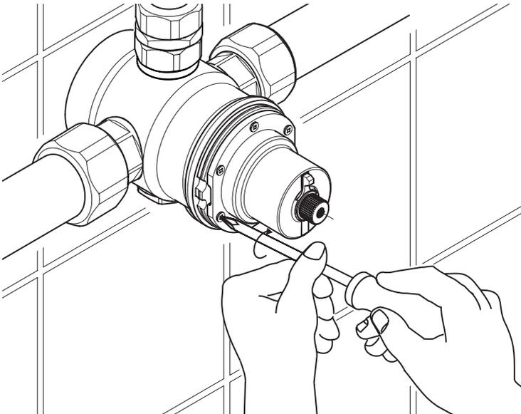
Install the six screws and tighten.
