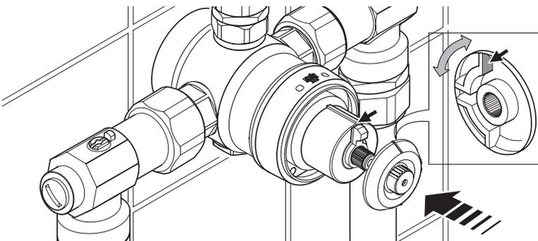
3. Once the desired maximum blend temperature is achieved, re-fit the hub without disturbing the spindle: Position the hub so that the hub stop comes up against the cartridge stop preventing any further rotation in an anti-clockwise direction. Check that blend temperature has not altered.
