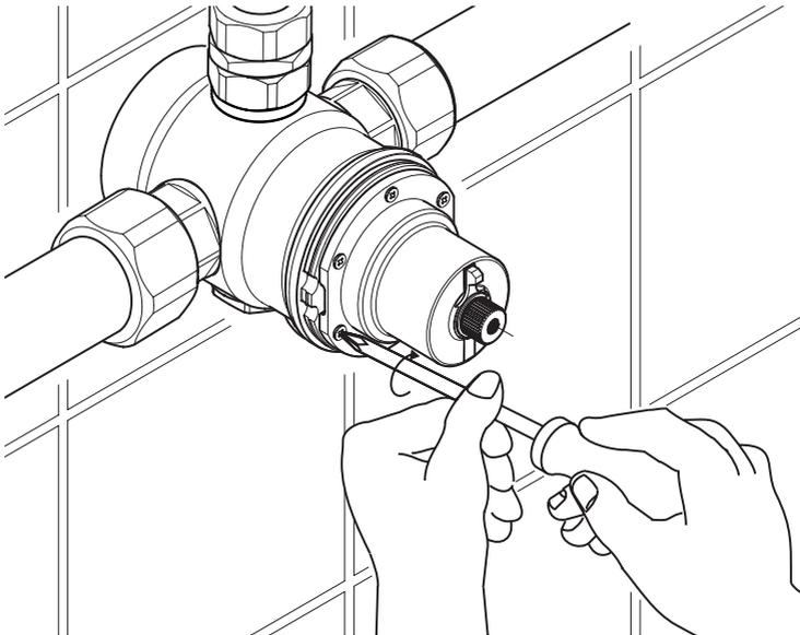
Install the six screws and tighten.
