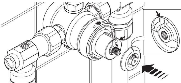
3. Once the desired maximum blend temperature is achieved, re-fit the hub without disturbing the spindle, positioning it so that the centre stop slot in the hub fits over the top of the cartridge stop, preventing any further rotation in either direction. Check that the blend temperature has not altered.
