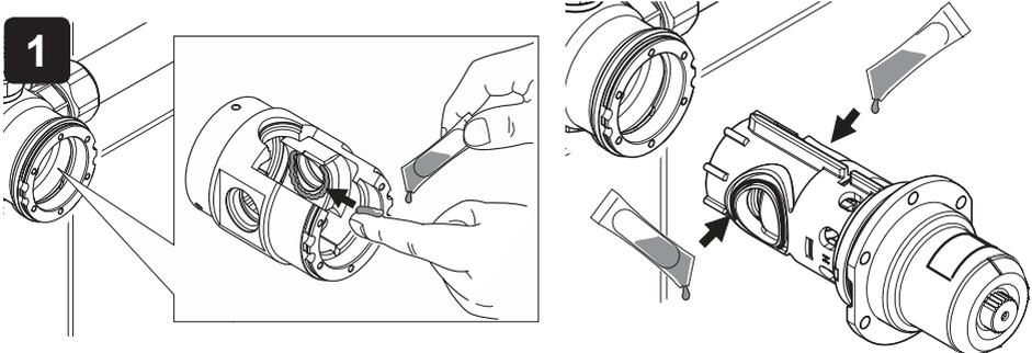
**Note!** Apply a small amount of silicone based grease to the top and bottom groove that the inlet seals fit to retain them whilst the cartridge is fitted. Fit the inlet seals to the cartridge and apply further grease to the seal faces and to the inside of the body as shown to aid insertion of the cartridge into the body.
