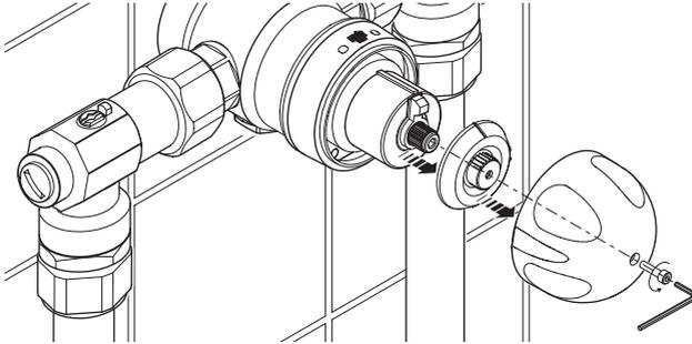
1. Remove the concealing cap, temperature knob and then the screw using the 3 mm hexagonal wrench (supplied). Remove the temperature knob and the hub.
