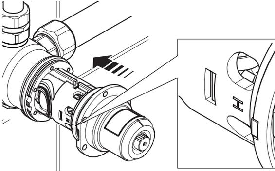
Identify which is the hot inlet to the mixing valve body, and align the cartridge assembly accordingly.
