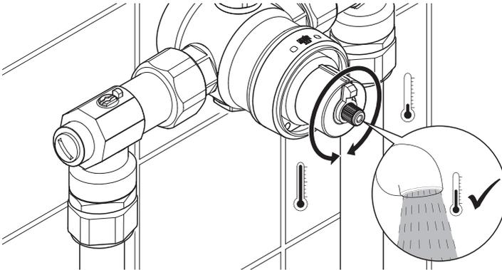
2. Rotate the spindle until required blend temperature is obtained at outlet point (**clockwise = decrease temperature, anticlockwise = increase temperature**).
