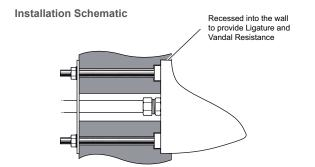
Note! Rear access is required for the installation of this product.
