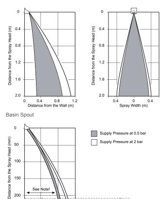
Note! The basin spout is designed for secure areas and is suitable where projection between the wall and the basin is kept to a minimum. Consideration must be given to the basin dimensions and positioning in relation to the spout spray projection, allowing for a minimum of 40 mm clearance over the rim of the basin
