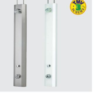
**Specify as: Rada PA-215TF Shower Panel Assembly (1.1613.046)** Ready to install satin finish stainless steel panel with hot and cold water pipe entry connection to a Rada 215-t3 TMV3 approved thermostatic mixing valve, with adjustable temperature selection, feeding a Rada TF503 push button timed flow control and Rada VR105 vandal resistant chrome plated shower head with integral strainer, flow regulator and with adjustable spray angle option.
